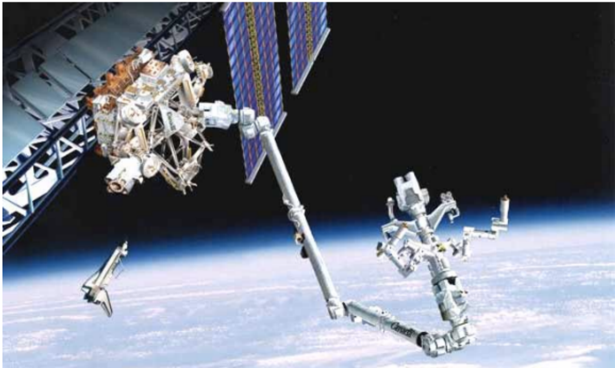
Fig-13 Special Purpose Dexterous Manipulator on the end of the Space Station Remote Manipulator
